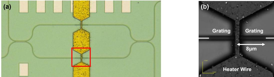
**Figure 2** (a) Micrograph of overall add-drop structure. (b) Confocal micrograph enlargement of the area in the red box from (a) showing the compact grating length of  $8\mu\text{m}$  each.
