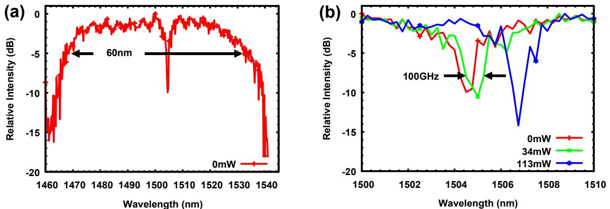
**Figure 3** Measured reflection spectra of the FP-based add/drop. (a) The stopband of the Bragg mirrors is 60nm wide, allowing a broad range of wavelengths to bypass the filter and exit at the Through port. (b) The passband of the FP cavity is 100GHz, transmitting only a narrow band to the Drop port. The wavelength of the FP passband can be tuned with the integrated metal heater.
