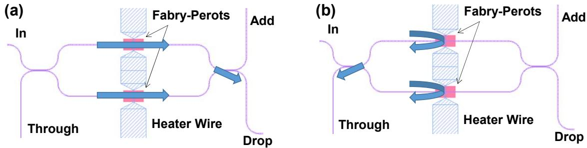
**Figure 1** Schematic and operating principle of the tunable wavelength add-drop filter. Two compact grating Fabry-Perot etalons are embedded in a Mach-Zehnder interferometer. (a) For resonant wavelengths, the signal goes to the Drop port. (b) For all non-resonant wavelengths within the stopband, light is reflected by the grating FP and sent to the Through port.
